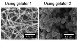
TiO<sub>2</sub> nanotubes TiO<sub>2</sub> nanoparticles
